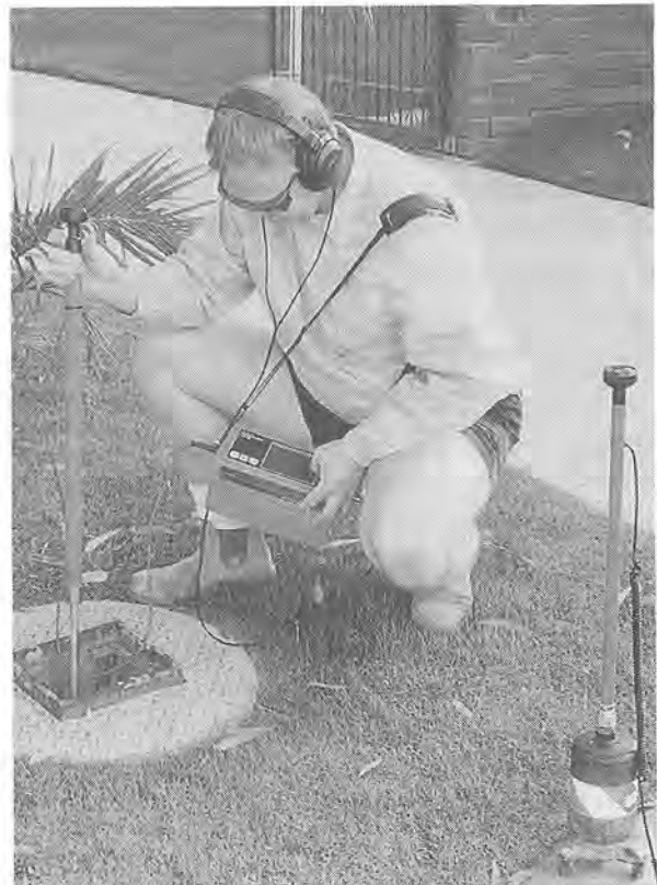
Council leak detection equipment
